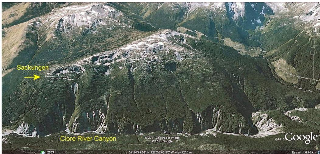
**Figure 10: Google Earth image looking to the southwest over the Clore River Canyon. Note the cirque shaped landslide scarps extending down to the Clore Canyon and the Sackungen (arrowed) that indicate slope deformation.**
