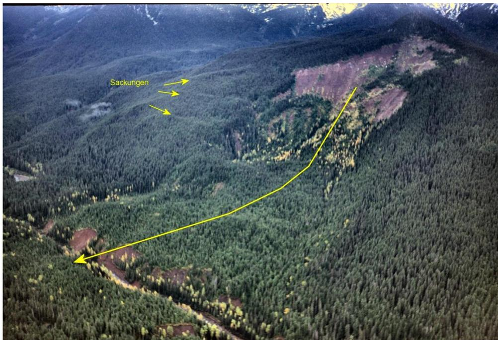
**Figure 8: A landslide in the red tuff volcanic bedrock, Kitnayakwa watershed, occurred about 220 years ago. The small arrows point to sackungen that indicate active slope movement that foreshadow a pending landslide.**
