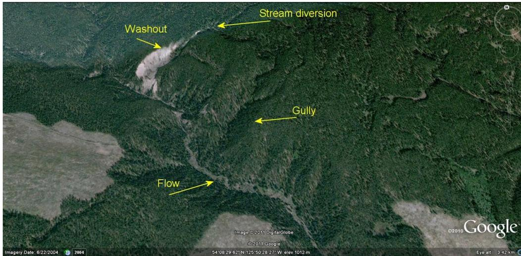
**Figure 2: Tchesinkut Creek washout-flow occurred in the early 1980s. Note the point of natural stream diversion; washout site; flow down Tchesinkut Creek; and, the similarity in shape of the washout-gully and the original gully down-cut through glaciofluvial-glaciolacustrine sediments.**
