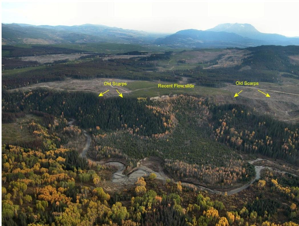
**Figure 6: A low gradient flow slide in advance-phase glaciolacustrine sediment at Houston Tommy Creek. Older landslide scarps are indicated with arrows.**
