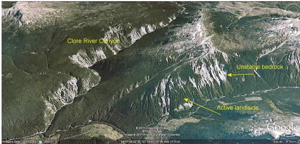
**Figure 9: Google Earth image looking east from the general location of Nimbus Mountain. The volcanic bedrock below 1200 masl is unstable and extensively gullied with visible landslide scarps and void of trees. The large active landslide is pushing the creek across the valley.**
