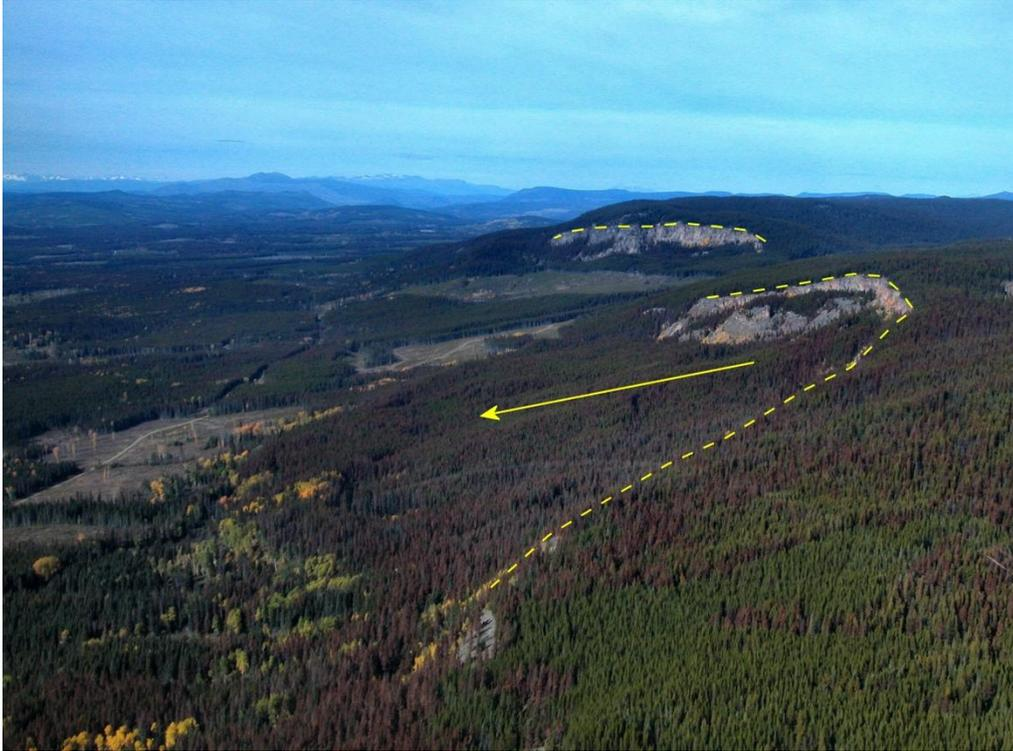
**Figure 5: Bedrock spread lead to catastrophic landslides along a 2.5 km scarp (photo lower centre to upper right) and a 1.3 km scarp (photo distance) on the ridge above Parrott Creek. The landslides involved up to 150 and 50 Mm<sup>3</sup> of material, respectively. The yellow dashed line delineates the landslides' headscarp. The arrow shows the direction of movement.**
